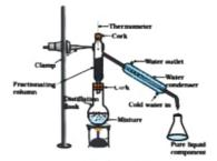
Petroleum is separated into paraffin wax, lubricating oil, diesel, kerosene, petrol and petrol gas by this method.
