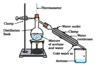
**Example:** When mixture of acetone and water is heated, acetone having lesser boiling point, boils and moves to delivery tube, within which it condenses back to liquid with the help of a condenser clamped to it. Thus, acetone is separated out in a beaker and water is left in the distillation flask.
