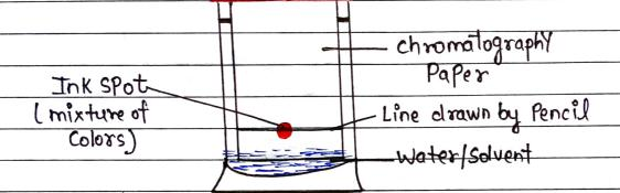
When water any suitable solvent moves up, the chromato -graphy paper ink with two different colours separates because both Colours are absorbed at different speeds.
